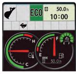
Checking DEF fluid level through Multi-function monitor.
