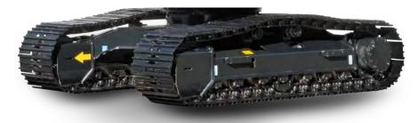
Reinforced undercarriage and increased crossbeam size and strength increase durability.
