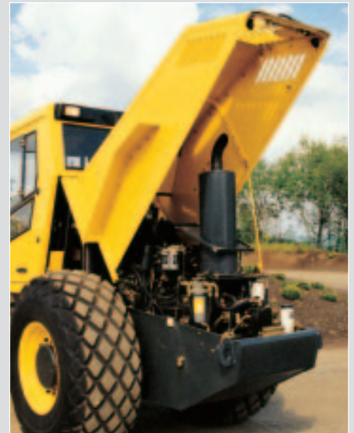
Large steel engine hood provides easy access to all service and maintenance points
