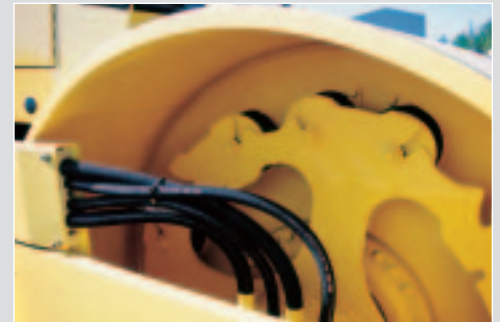
Individually changeable rubber buffers with no special tools or disassembly of the drum required
